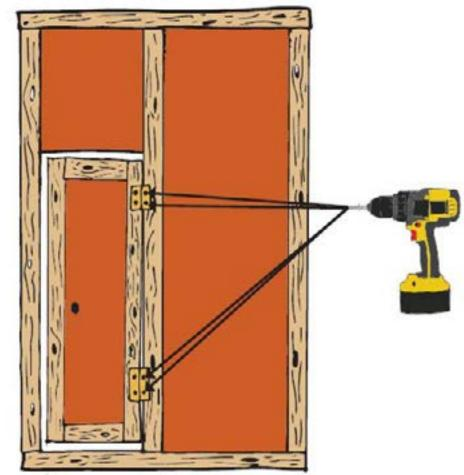
You then will have to attach the door by the hinges by screwing into the support that you have inserted into the panel.
