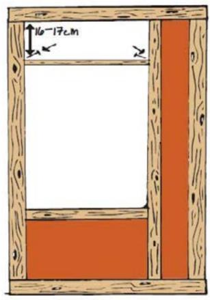
You now want to measure between timber shell and the vertical support to make the first row. Cut the wood into the measurement you get and repeat another three times. It should be approximately 72cm. You want to measure approximately 16—17cm as this is the typical size of A5 but gives a little leeway. You then want to attach them by using a hammer and nail at either side.
